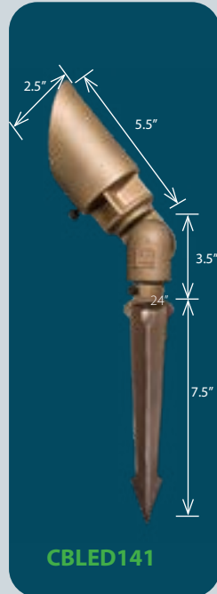
LED Bullet CBLED141 Solid bronze body, shroud, and 7.5" stake, LED module has two light levels, 25' #16-2 No-Ox® Wire lead (equivalent to 35W & 50W halogen)
