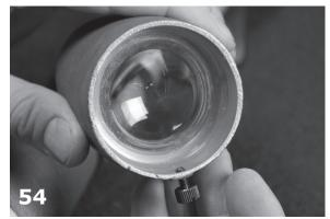
Before applying shroud, retract set screw so it does not extend past inside shroud surface.
