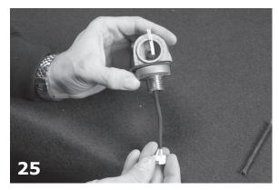
Insert socket wire into knuckle top.
