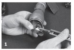
Remove shroud and heat reflector.
