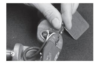
Cut wire junction on wire-side of crimp.
