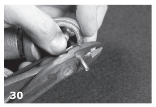
Using crimp tool, crimp barrel over wire ends.
