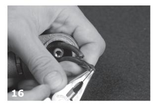
Using pliers, remove old heat shrink.
