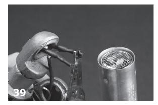
Using plier, compress heat shrink past crimp.
