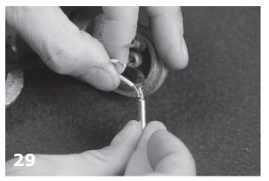
Slide crimp barrel over bare wire ends.
