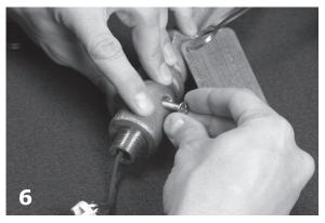
Unscrew and remove knuckle screw.
