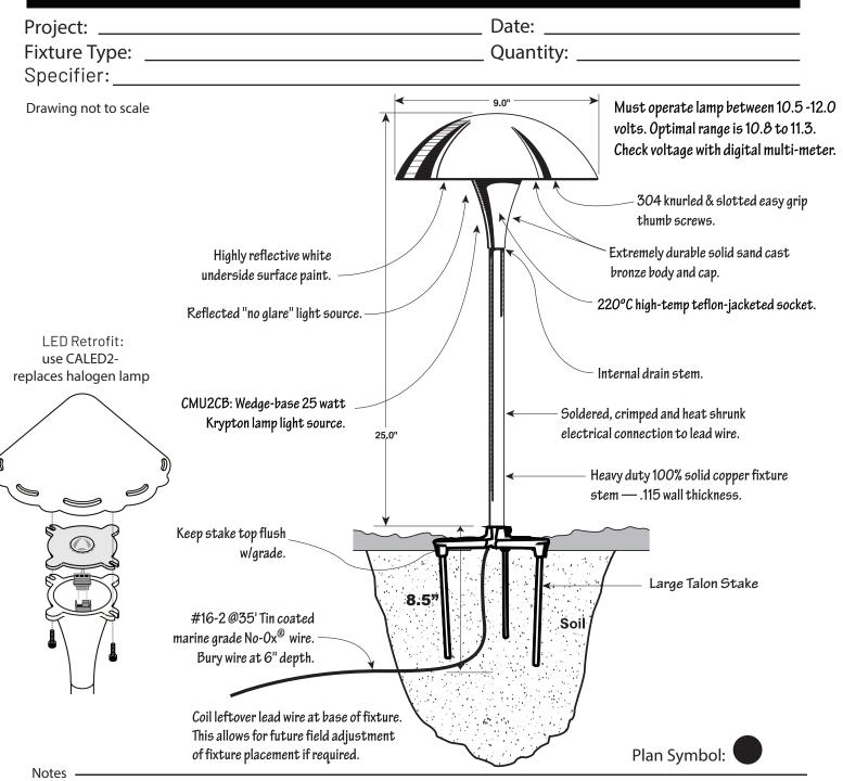
• CMU2CB: Requires S8 Wedge Base Lamp (incl. 25w) Max. lamp rating 35 watts
