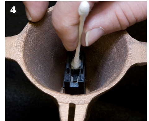
4 Apply thin layer of grease to a clean cotton swab. Rub a small amount of grease on each contact. Do not allow grease to contact plastic between contact pairs.*
