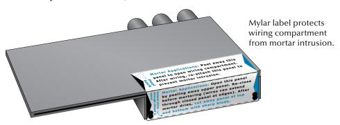
Label can be peeled back for wire installation then re-sealed prior to mortaring.
