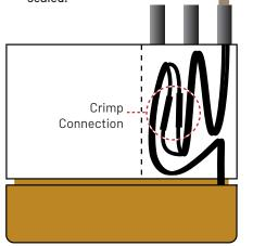
Up to three wires can enter module to enable looping through fixtures.
