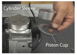
Place the retainer plate into a new piston cup making sure that the lip of the piston cup faces up.
