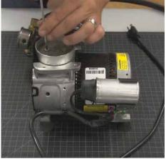
Flip the new valve plate over to install the new cylinder o-ring.
