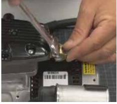
Using a T25 Torx wrench, remove the four screws on the top of the head assembly.
