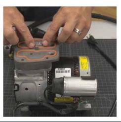
Align the head cover on top of the valve plate and install the 4 screws to secure the head cover to the valve plate. We recommend going back and forth between screws to ensure the screws are securely in place. Be sure not to over tighten (Recommended Torque: 47-50 in lb).
