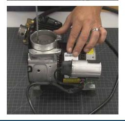
Remove the cylinder sleeve and worn piston cup and discard. Place the new piston cup beneath the retainer plate with the lip of the piston cup facing up.
