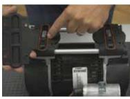
Install the six screws to secure the head covers on the valve plates. Leave the inner two screw holes open. We recommend going back and forth between screws to ensure the screws are securely in place. Be sure not to over tighten (Recommended Torque: 47-50 in lb).
