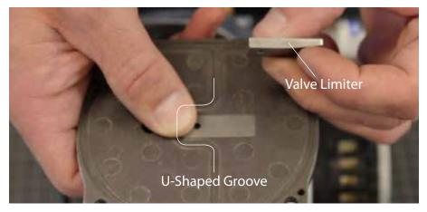
Install the leaf valve, ensuring the leaf valve and limiter are located on the side opposite of the o-ring gasket. Place the leaf valve with the limiter on top in the "U" shaped groove on the valve plate and cover the hole. Ensure the curved portion of the limiter rests on the leaf valve.
